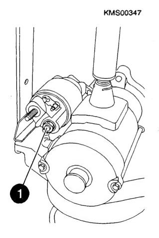
STARTING MOTOR ASSEMBLY Sealing starting motor Starting motor must be sealed following assembly. This involves liberally applying nitrocellulose combination lacquer to starting motor in marked area (x) as shown.
